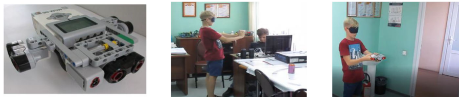
Fig. 7 Arranging of sensors and the unit for controlling the first prototype of the electronic guide for blind people
